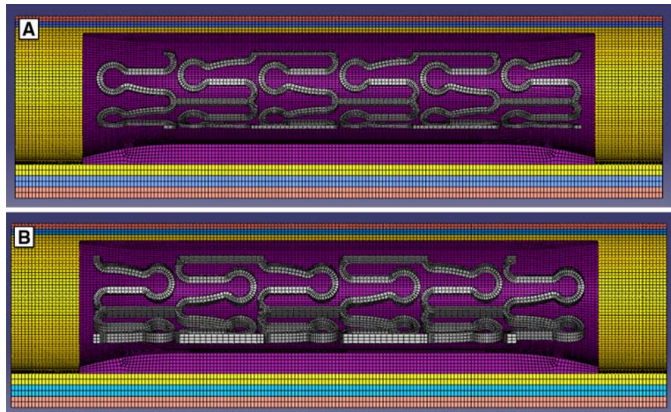
Fig. 1 Finite element models of the atherosclerotic coronary arteries with crimped a multilink thin and b multilink thick stents
