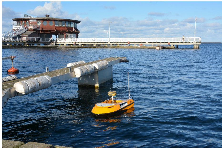
Figure 2. OceanAlpha USV SL20 during bathymetric surveys in Puck marina.
