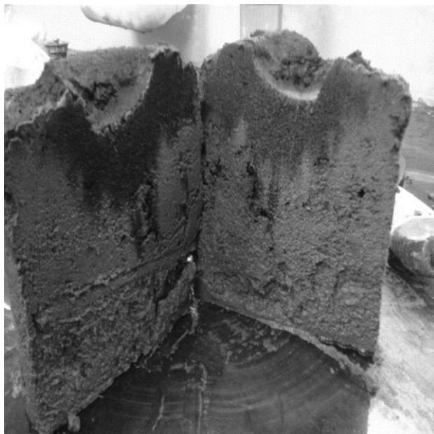
Figure 5. Visual analysis of the dye transport pathways: retardation in connected macropores that are not connected to the bottom of the soil sample
