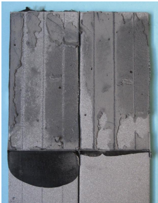
Figure 25- Fracture surface of a joint without fibers (second trial).
