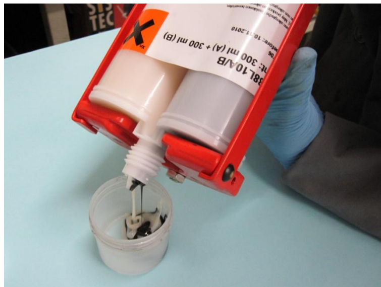
Figure 44- Adhesive's extraction using an adhesive applicator gun.
