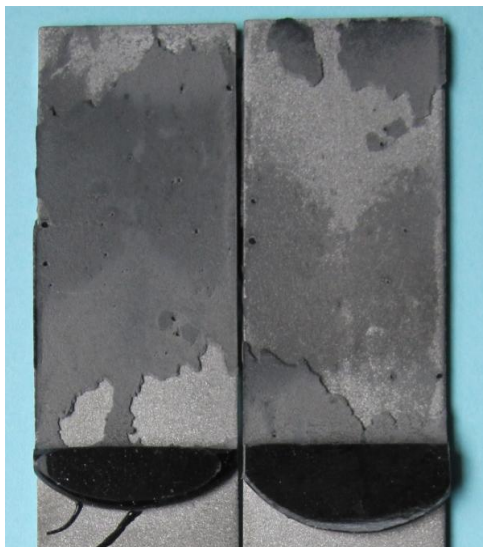
Figure 21- Fracture surface of a joint without fibers (first trial).
