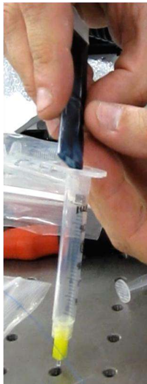
Figure 52- Epoxy is poured into the syringe.
