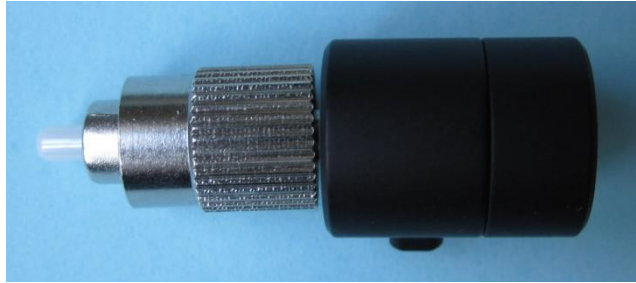
Figure 60- Universal bare fiber terminator and FC connector.
