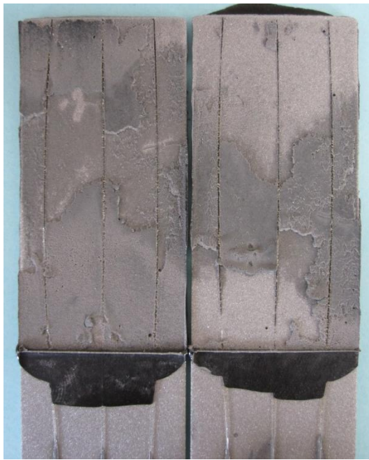
Figure 34- Fracture surface of a joint (fourth trial).
