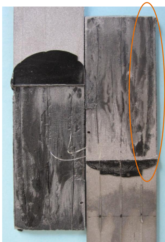
Figure 30- Fracture surface of a joint (third trial).
