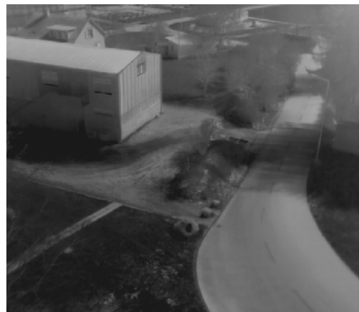
Figure 1: Example for a thermal image acquired by a thermal camera FLIR Tau 640.
