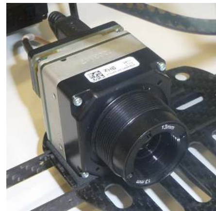
Figure 4: Thermal camera FLIR Tau 640; focal length 13mm.
