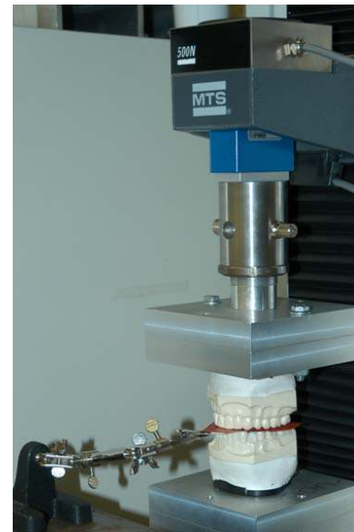
Fig. (2). MTS testing machine - closed with casts intercusped and articulating paper horseshoe interposed.
