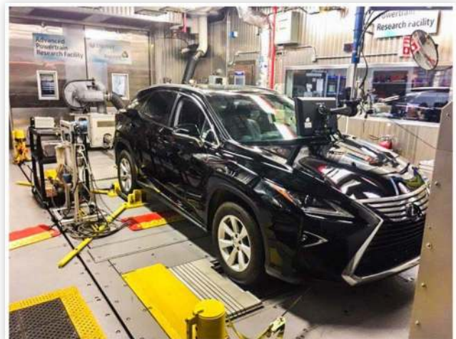
FIGURE 2 2016 Lexus RX350 test vehicle on APRF dynamometer for testing.
