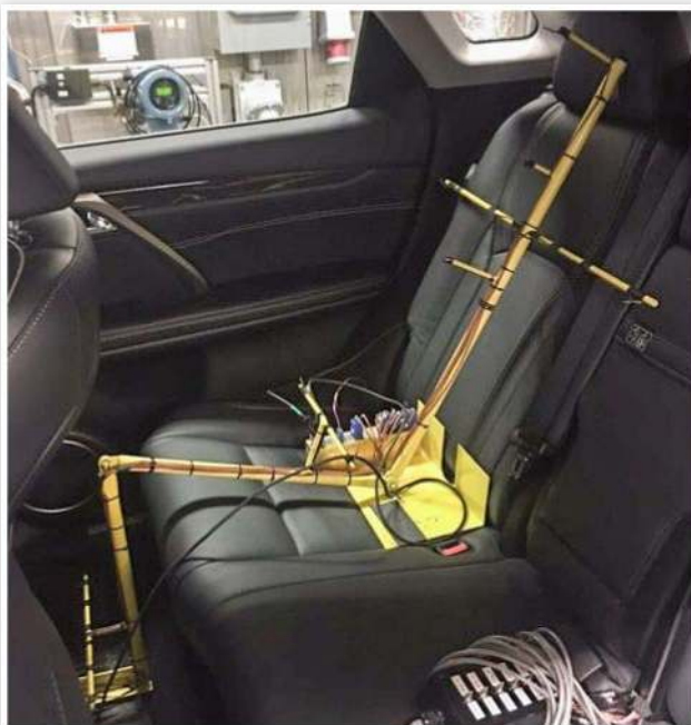
FIGURE 3 Passenger side rear seat mannequin thermocouple instrumentation.
