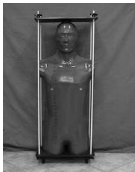
Figure 1. Alderson Rando phantom.
