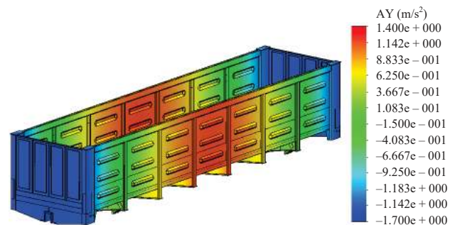
Fig. 9. Distribution of acceleration fields acting on the bearing structure of the body of a semi-wagon under a viscous interaction with the deck of a railroad ferry (side view)
