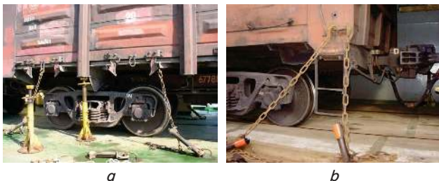
Fig. 1. Fixing a semi-wagon relative to the deck of a railroad ferry: a – via the elements of a hatch cover lock; b – via a towing bracket
