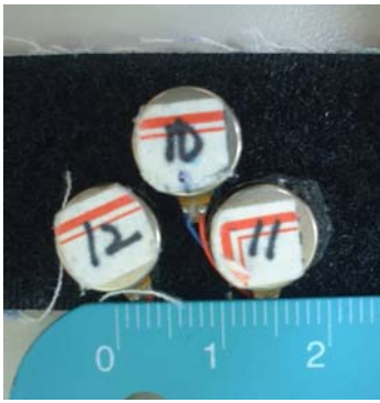
Figure 6: 3 element vibrotactile array used in intensity study.
