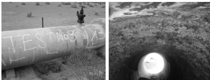
97 Figure 1 – External and internal views of a section of pipe with internal damage
