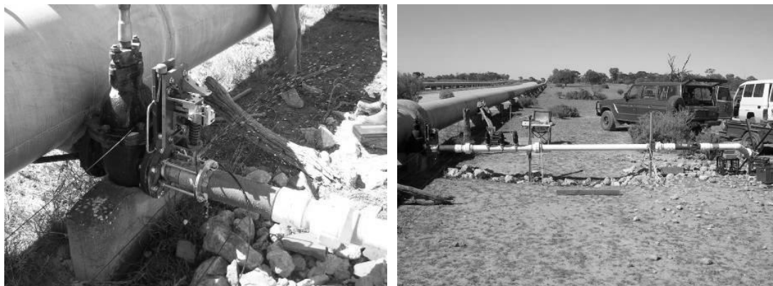
432 Figure 4 – Transient Generator, PN16 PVC Discharge Pipe, Inverted Foot Valves and 433 Paddle Wheel Flow Meter Locations
