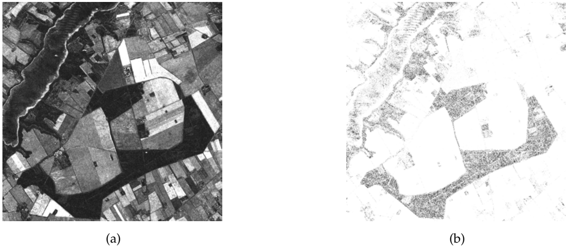
Figure 5. (a) -2\rho \ln q_{obs} for full polarimetry (stretched linearly between 0 and 300), and (b) P(Q \geq q_{obs}) , both based on data from March to July. In both images low values (dark tones) correspond to no change.
