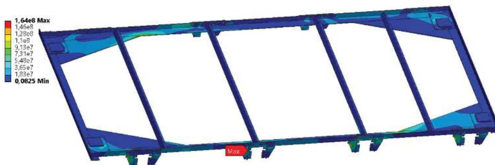
Fig. 7. The distribution of equivalent stresses in a semi-frame for a container (general view)
