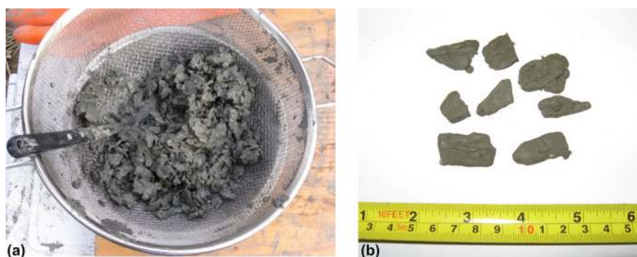
Figure 3. Evaluation of core cuttings as an alternative sample source for DVE-LS: (a) sieved chip samples after washing, and (b) wiped chip samples (typically 25 × 15 mm) prior to placement in Ziploc™ bags.
