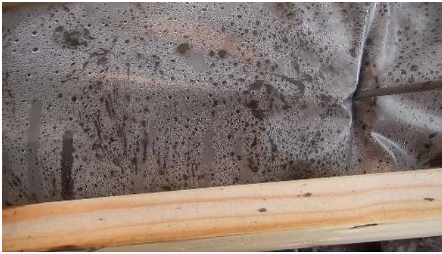
Figure 7. Vapour condensation on the inside of plastic sampling sleeve at ground surface. Core temperature at ground surface was 85 °C.
