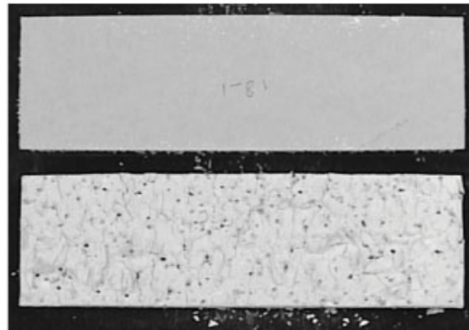
Images of Gypsum Samples Before and After Oven Drying
