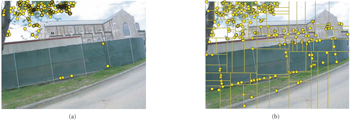
FIGURE 2: The goal is to select 256 representative features in the image. (a) The 256 strongest features are concentrated in a small area in the image—more than 95% are located in the tree at upper left. (b) After applying the k-d tree partition with 128 leaf nodes, the features are more uniformly spatially distributed.
