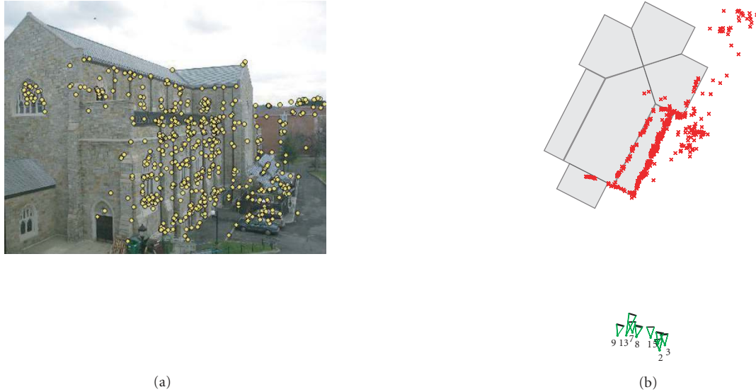
FIGURE 8: Camera calibration results for a prominent building in the scene. (a) Original image 2, with detected feature points overlaid. (b) The 3D reconstruction of the corresponding scene points and several cameras obtained by the distributed calibration algorithm, seen from an overhead view, with building shape manually overlaid. Parallel and perpendicular building faces can be seen to be correct. Focal lengths have been exaggerated to show camera viewing angles. This is only a subset of the entire calibrated camera network.
