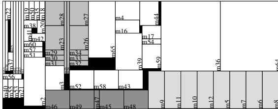
Fig. 18. Result of “biasynth_2p4g” obtained by the approach of this paper. (Time: 5.6min, Area usage: 104.96%)
