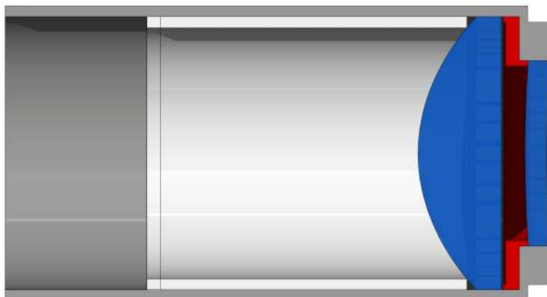
Figure 5.10: Mount for the lenses of the focusing objective. The right distance between the aspheric lens and the meniscus lens is set by a spacer (red) which also centers the meniscus lens with respect to the optical axis. The aspheric lens is centered to the same axis via a tube which is fixed by means of a retaining ring.
