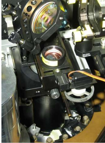
Figure 5.14: Microtrap setup. The laser beam which is focused to create the microtrap passes a dichroic mirror from above and enters the objective (black tube). To prepare the reservoir of cold atoms a motorized mirror is inserted into the beam path for operation of the magneto optical trap.
