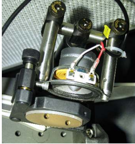
Figure 7.6: To excite an atom in the ground state to the first excited state with frequency \omega_{01} the symmetry of the wave function has to change which requires an operator with odd symmetry. We realize this operator by translating the center position of the potential by shaking the micro-trap mirror with a loudspeaker.
