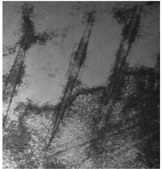
Fig. 3—TEM micrograph of NiTi overaged (823 K, 1.5 h) specimen [123] showing the precipitates and dislocations (after thermal cycling).
