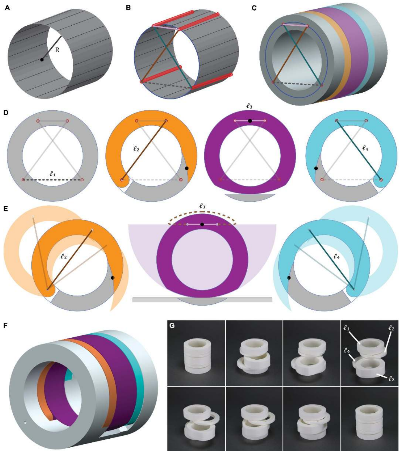
Fig. 7. Steps for the creation of a developable mechanism, illustrated using a Chebyshev straight line mechanism integrated with a cylinder. (A) A cylinder with radius R selected as the base surface for the Chebyshev mechanism. (B) The ruling lines (red) that will serve as joint axes and the corresponding linkage skeleton. The ground link ( l_1 ) is dashed, while the remaining links are solid. (C) Applied thickness and selected link layers in the surface. (D) The geometry of each of the link layers, accompanied by their corresponding skeleton links, with l_1 (gray), l_2 (orange), l_3 (purple), and l_4 (blue). (E) The process used for defining link geometries. Motion analysis informs link shapes that avoid interference between the links. (F) CAD model of the developable mechanism. (G) Physical prototype with links labeled, demonstrating the motion of the linkage.
