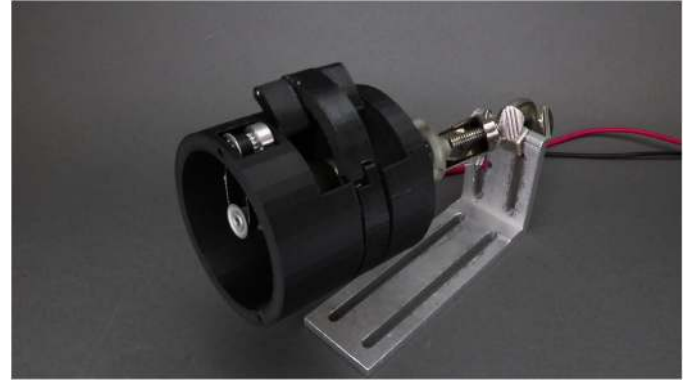
Movie 3. Motorized 4R cylindrical developable mechanism. A possible walking or active-gripping motion is demonstrated.
