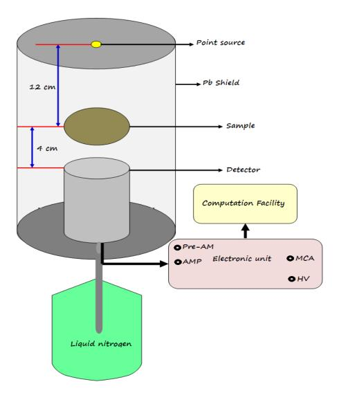
Figure 2. The geometry of the experimental work.
