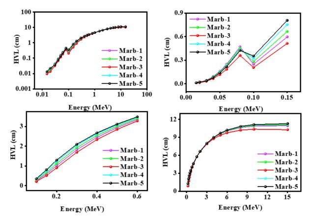
**Figure 6.** Illustration of the HVL of the prepared composites (polyester/waste marble/PbCO<sub>3</sub>/CdO) against incident photon energy.
