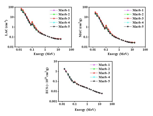
**Figure 7.** The theoretical values of LAC, MAC, and ECS of the prepared composites are within the energy limit of 0.015 MeV to 15 MeV.
