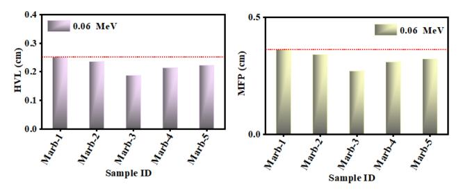
Figure 10. The value of the HVL and MFP of the prepared composites at energy 0.06 MeV.
