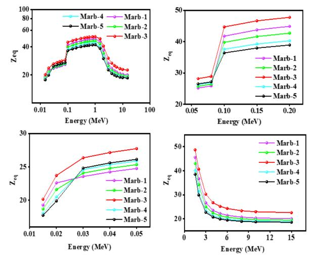
**Figure 11.** Illustration of the equivalent atomic number ( $Z_{eq}$ ) of the prepared composites (waste marble/polyester/PbCO<sub>3</sub>/CdO) against incident photon energy.
