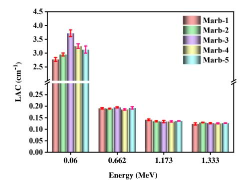
**Figure 3.** The demonstration of LAC of the prepared composites at energy 0.06 MeV, 0.662 MeV, 1.173 MeV, and 1.333 MeV.
