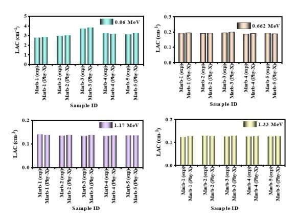
**Figure 4.** Demonstration of the deviation of the *LAC* values between the experimental and Phy-X software values.
