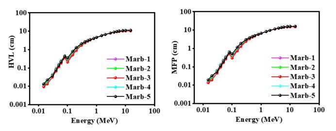
**Figure 9.** The theoretical value of the HVL and MFP of the prepared composites within the energy limit of 0.015 MeV to 15 MeV.
