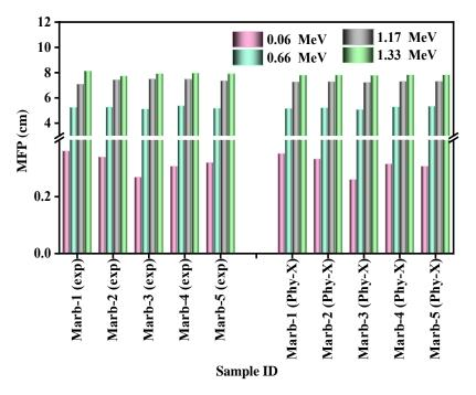
**Figure 8.** The comparison between the experimental and theoretical values of the MFP of the prepared composites.
