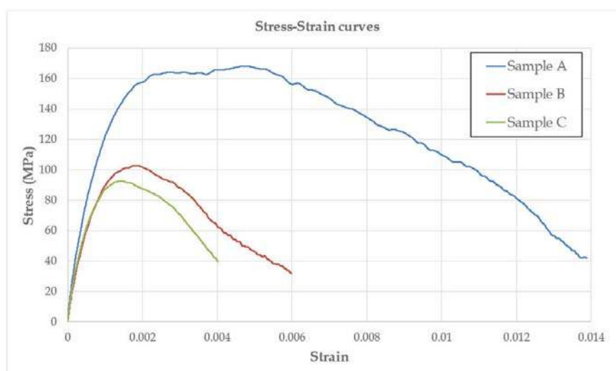
Figure 6—SHPB true stress-true strain curves using one example from each of the mineral texture types, i.e. shale (sample A) against the two different polymetallic ore samples (B and C)
