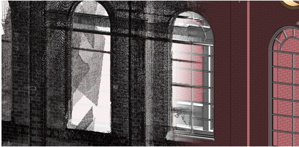
Figure 7: Using Scan to BIM methodologies for geometric modelling existing building
