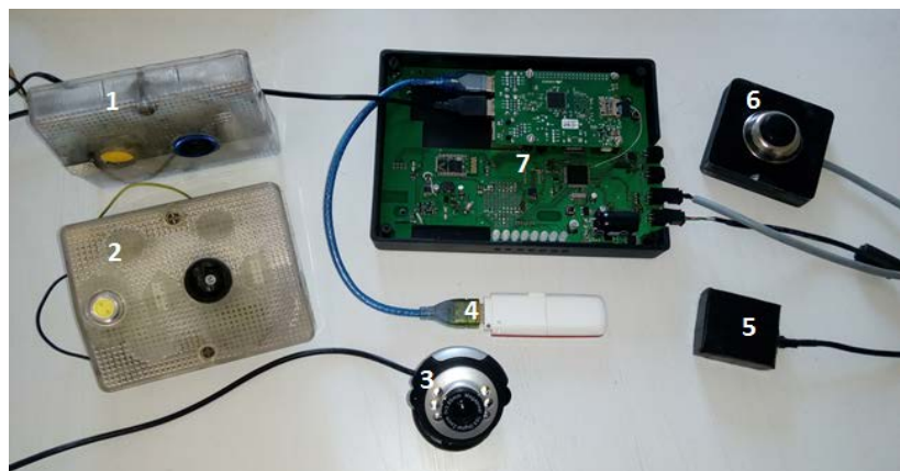
Fig. 7. Main components of the designed device (1 – plafond with front camera, 2 – plafond with rear camera, 3 – certificate camera, 4 – 3G modem, 5 – GPS module, 6 – certificate button)
