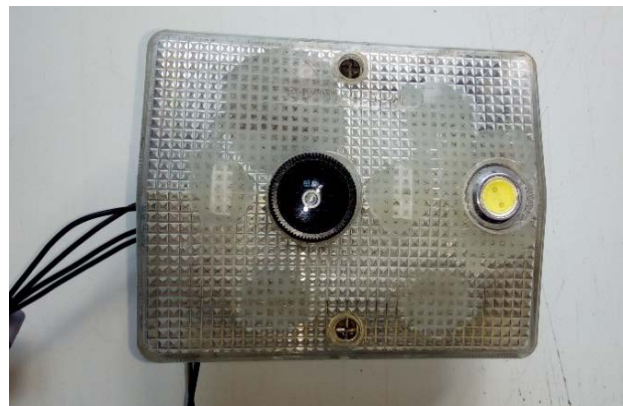
Fig. 6. Plafond with a camera
