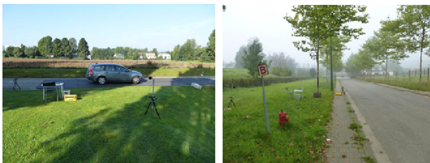
Figure 9 – Controlled Pass By measurements on the Sterrebeek II test track and on an ordinary dense asphalt concrete pavement (reference) (pictures by A. Bergiers, BRRC)
