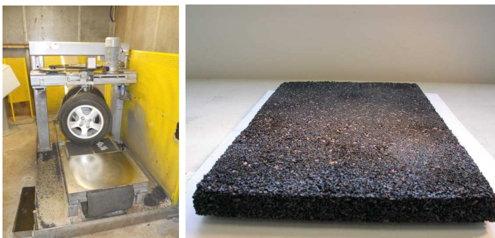
Figure 1 – The Aachener Ravelling Tester (ARTE, left hand side) and a PERS test slab after being exposed to the test
