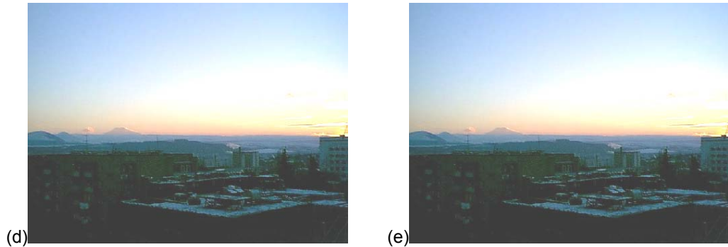
Fig. 6. a) The source Image, b) the result image after histogram equalization with using HSI color model, c) the result image after histogram equalization with using RGI model, (d) the result of brightening with using HSI model, (e) the result of brightening with using RGI color model.
