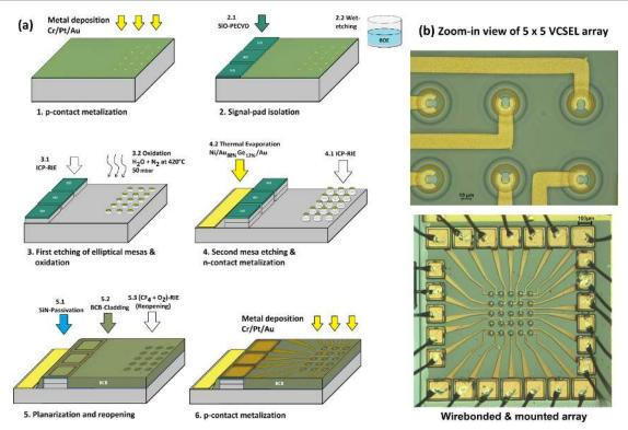
Figure 2. (a) Schematic overview of the sample fabrication process as described in section 2. (b) Microscope images of the finished VCSELs and the fully wirebonded and mounted array.
