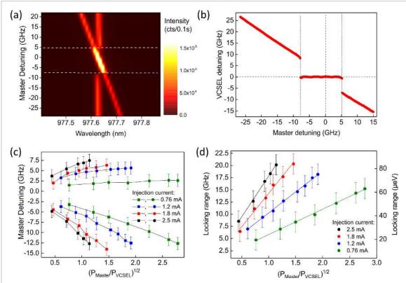
Figure 4. (a) 2D intensity map of VCSEL emission under optical injection by an external tunable laser for a bias current of 1.2 mA and an injected power of 0.87 mW. (b) Relative emission frequency of the VCSEL acting as slave laser as a function of the master laser detuning. (c) Power dependent measurement of the boundaries of the locking area. (d) Injection power dependent locking range for different injection currents.
