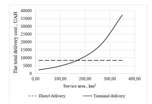
Fig. 5. Graph of the total cost dependence on service area
