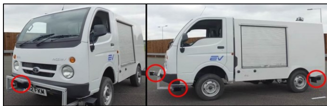
Fig. 2. Tata ACE autonomous vehicle platform showing LIDAR sensors.
