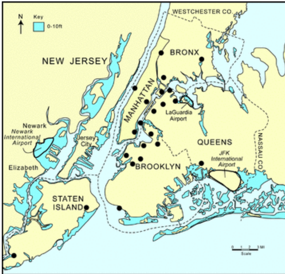
Figure 7. Locations of New York City power plants relative to 10-foot elevation contour. Source: NPCC, 2010
