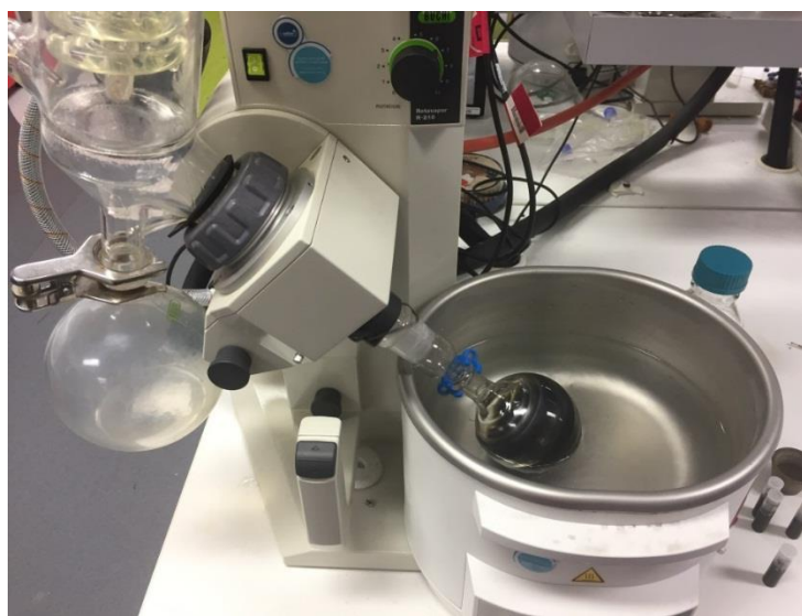
Figure 5.1 Rotary evaporation used to make viscous PUHC (contained in round bottom flask in the water bath) at 25 °C, 90 rpm in 10 mbar.
