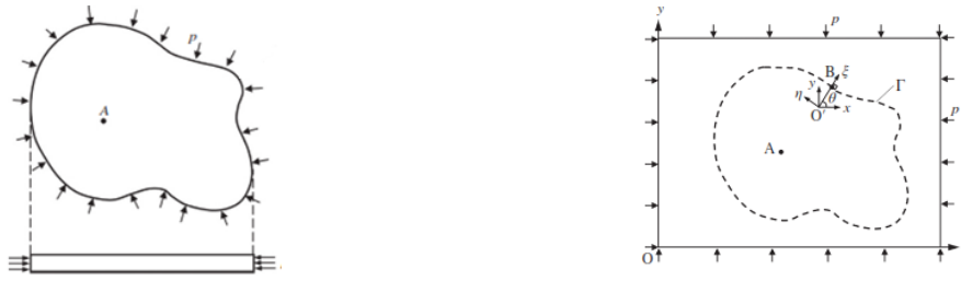
a) A plate under in-plan constant stress. b) Visualizing the plate as a part within a larger.
