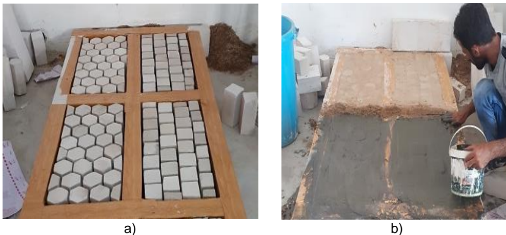
Fig. 8: Specimens manufacturing process.
