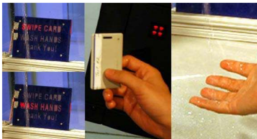
Figure 2.3 – Clean Sink showing indicator (left), RFID reader (middle) and sink (right) from [7], Figure 3.
