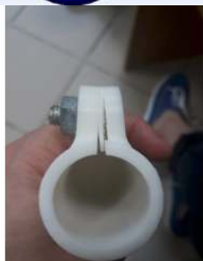
Fig. 10. Delamination of the handle
