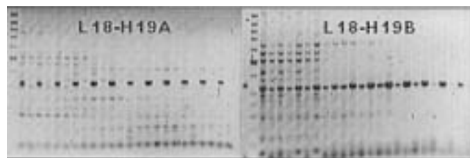
Fig. 4. Comparison of single nucleotide polymorphism (SNP) primers developed to differentiate cucumber lines H-19 and G421. Primers designed on a 5-bp polymorphism (L18-H19A) vs. a 2-bp polymorphism (L18-H19B). Lane 1 contains a 100-bp ladder, and the remaining lanes contain paired DNA of lines H-19 and G421, which underwent PCR in ascending 1.8 °C intervals from 45 to 65 °C.
