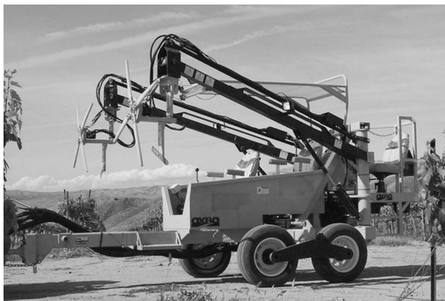
Fig. 5. Korvan™ Vineyard System chassis equipped for shoot thinning. The speed of the tractor used to pull the chassis and the speed of the thinner paddles can be adjusted so that the thinner leaves the desired number of shoots per foot of cordon, depending on cultivar and vigor (photo courtesy of OXBO International Corp., Clear Lake, WI).
