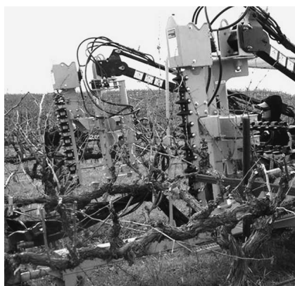
Fig. 4. Korvan™ Vineyard System chassis with shear pruning attachments on both right and left sides. This configuration allows the tractor-pulled unit to prune facing sides of adjacent rows. Shown working in Vitis vinifera at French Camp Vineyards, Santa Margarita, CA (photo courtesy of OXBO International Corp., Clear Lake, WI).
