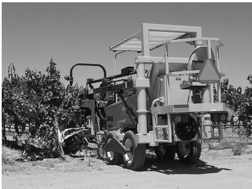
Fig. 6. Korvan™ Vineyard System chassis equipped with grape thinning attachments for bottom thumper fruit thinning on 2-ft (0.6-m) lyre and quadrilateral-trained vines. Shown working in Vitis vinifera at French Camp Vineyards, Santa Margarita, CA (photo courtesy of OXBO International Corp., Clear Lake, WI).
