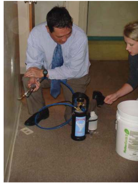
Fig. 6. The HHRA staff and administration attended a hands-on seminar where they were taught how to apply the perimeter diatomaceous earth barrier using a Cyclone Power Duster.
