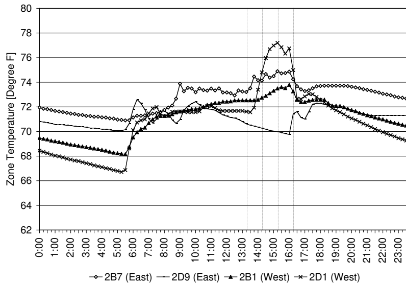
Figure VII-20. GSA – South Tower 2nd Floor Zone Temperature
