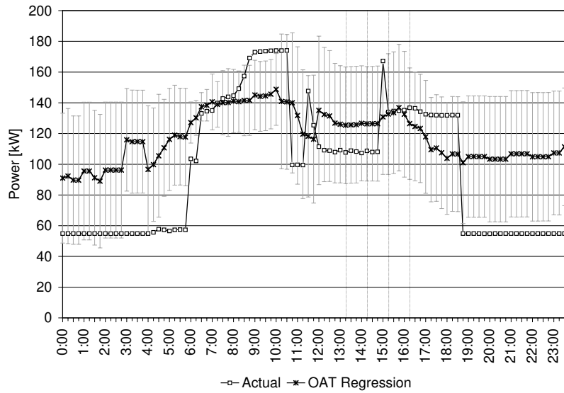
Figure VII-11. GSA – Pump Power and OAT Regression Model
