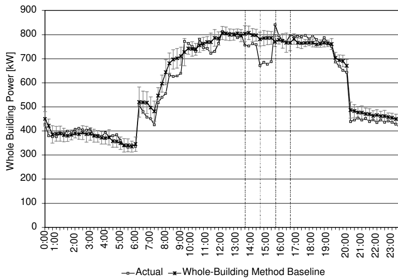
Figure 4-33. UCSB – Whole Building Power and Baseline (Whole-Building Method)
