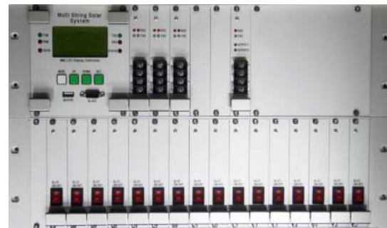
Fig. 7. Multi-string power balancing system.
