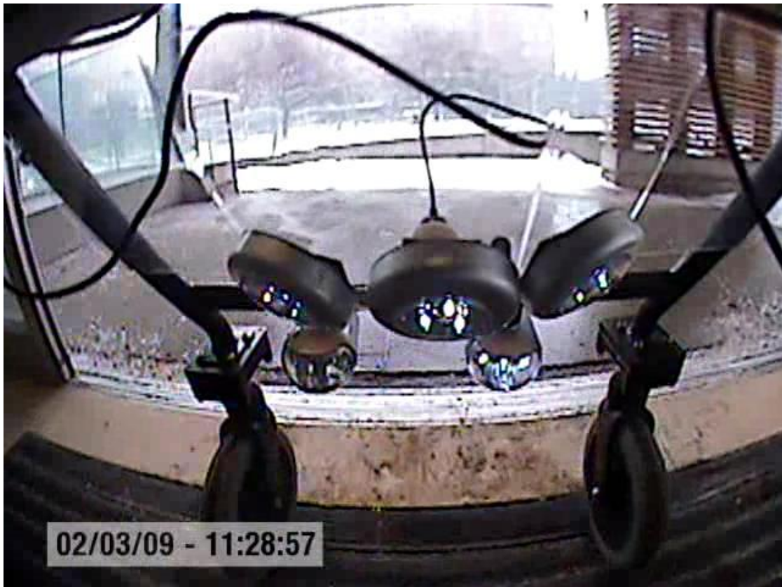
Figure 5: Screen capture from a video record of the scene camera aimed at the upcoming environment. Note that the front two wheels of the rollator are captured in the view to maintain a frame of reference.
