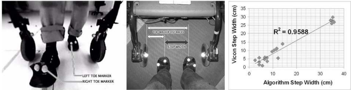
Figure 3: Development of spatiotemporal foot placement measurement method. View of feet and markers from foot placement camera (left panel). Step width calculation (middle). Comparison of step widths calculated by the algorithm and Vicon (right).
