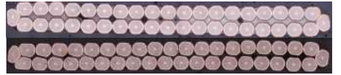
FIG. 6. Cross section of the rectangular (top) and keystoneed (bottom) cross sections of the demonstrator dipole cable.
