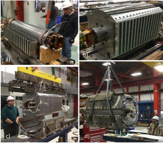
Fig. 5. The cold mass assembly steps: a) insertion of coil block inside the half-yoke; b) yoke clamping with I-clamps; c) insertion of clamped yoke inside the half-skin; d) cold mass inside tooling is moving to press for skin welding.
