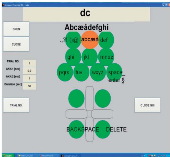
Figure 9. The Matlab® based visual feedback used in the experiments. The given character string to be typed is shown with the currently desired character in capital. In the text field above, the characters typed by the subject are displayed. Correctly typed characters are shown in capital. A figure below the text field shows the position of the characters on the keypad area of the ITCI. As default, all sensors were marked with a green circle. When the activation unit was placed at a sensor/character for less than the time D1, the circle around the character turned yellow, and the character was temporarily typed at the cursor in the text field. When D1 was exceeded, the colour turned from yellow to red and deactivation of the sensor resulted in sustained typing of the character in the text field after which the cursor moved one step forward to provide feedback for the next character to be activated by the subject. If no deactivation occurred within the time D2, the next character related to the activated sensor was displayed.
