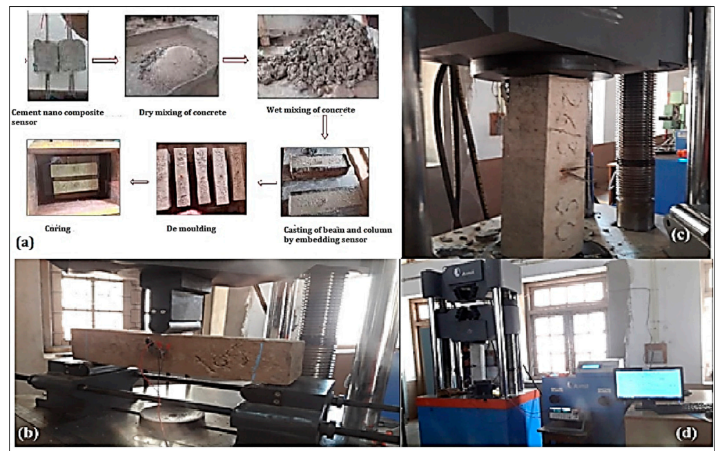
Figure 7. (a) Preparation of structural component beam and column by embedding cement-based sensor (b) Test set up for flexural test on beam (c) Test set up for column subjected compression load (d) UTM of 100-ton capacity.
