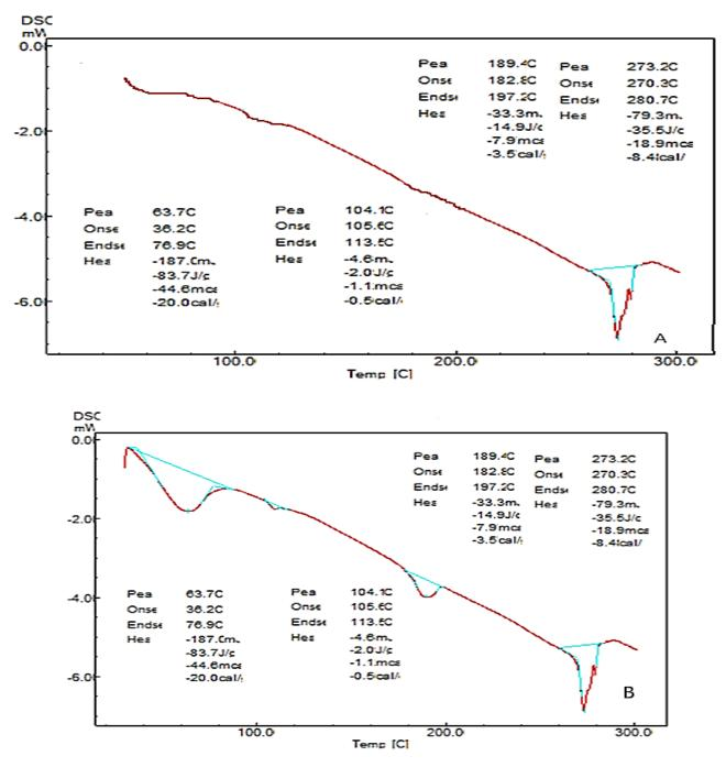
Figure 5. DSC thermograms of (A) pure drug and (B) nanocarrier.
