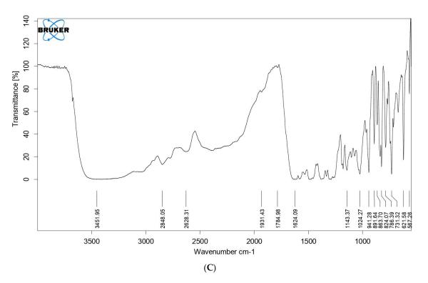
Figure 6. FTIR with characteristics peaks of (A)  $\beta$ -TCP (B) Pure drug (C) Nanocarriers' formulation.
