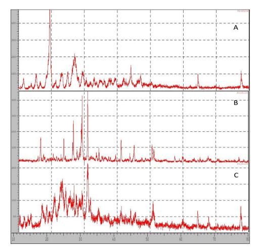
**Figure 7.** X-RD pattern of (**A**) Pure drug (**B**) β—TCP, (**C**) Nanocarriers (F1).
