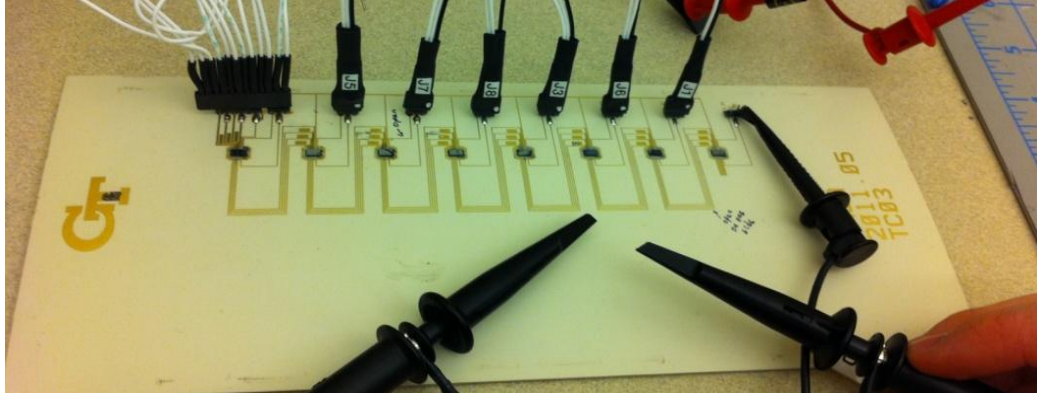
Figure 4.22: Digital test board populated with eight T/R modules.
