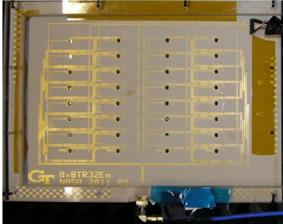
Figure 4.25: Fabricated array populated with 32 T/R modules and connected for near-field chamber measurements.
