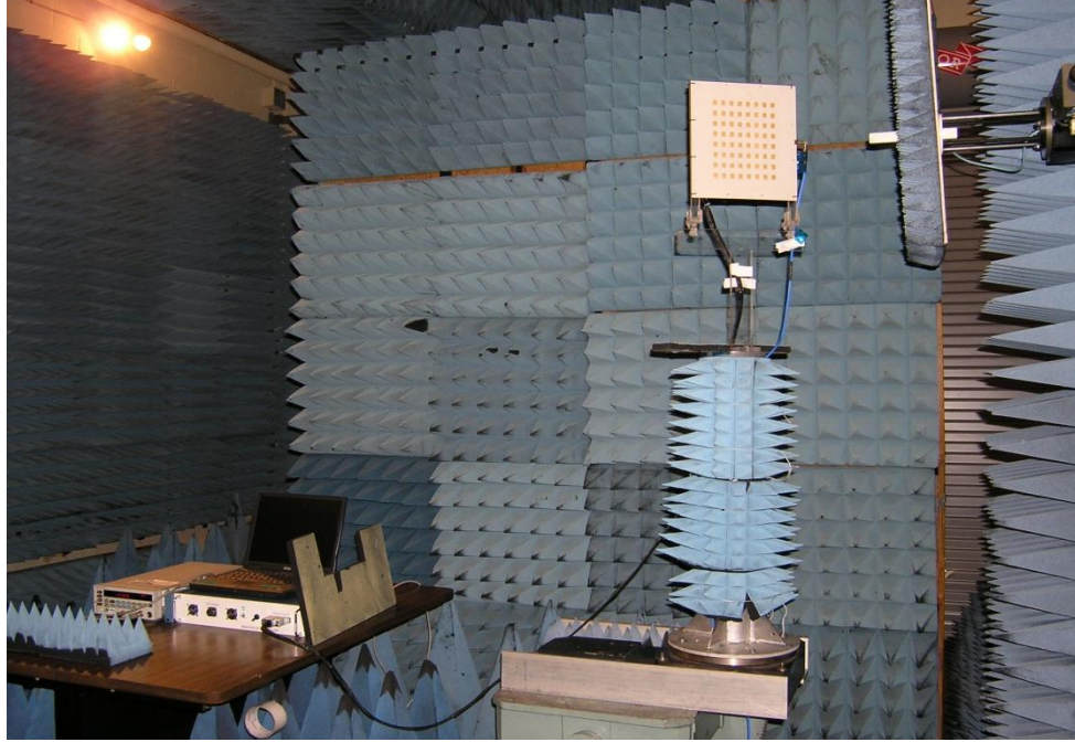
Figure 4.26: Near-field range chamber test setup for characterizing the antenna radiation patterns.
