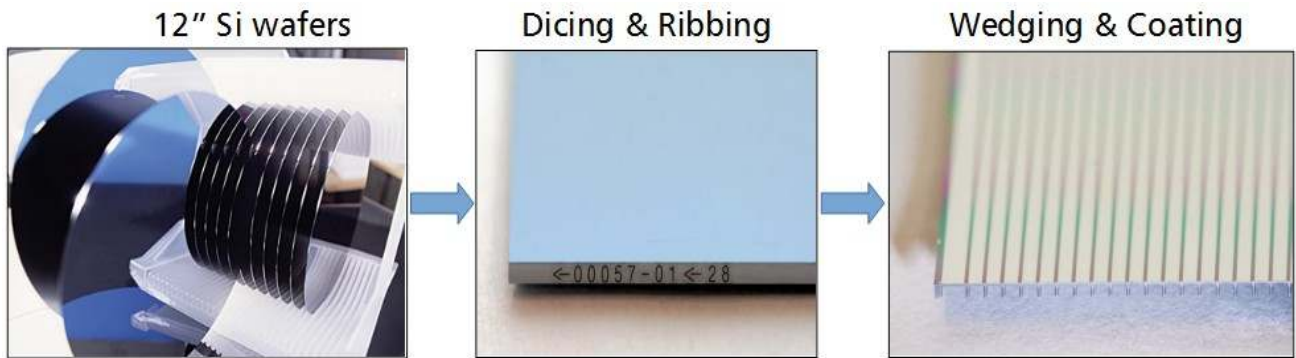
Figure 1. Overview of process flow for production of SPO mirror plates.
