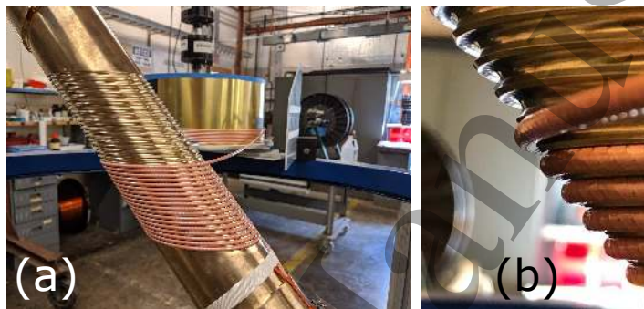
Figure 4. (a) Winding Layer 2 using the existing winding table [31]. (b) CORC ® wire enters the half-depth groove.
