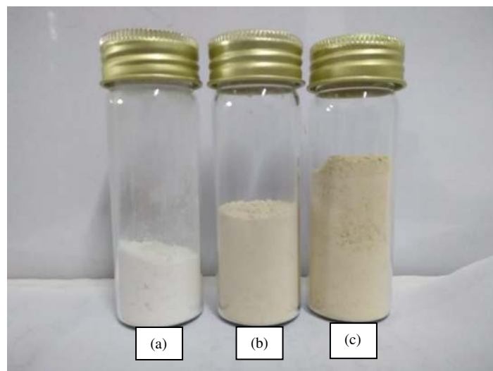
Figure 5 Palm Powder obtained from different Spray drying conditions (a) Maltodextrin aided spray-dried palm powder (b) Gum Arabic aided spray-dried palm powder (c) Combined Additive aided spray-dried palm powder
