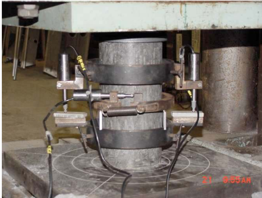
Figure 4.18: Test Set-Up for Measuring the Elastic Constants
