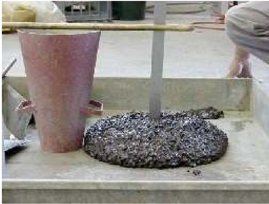
Figure 3.11: Slump Measurement of Fresh Concrete
