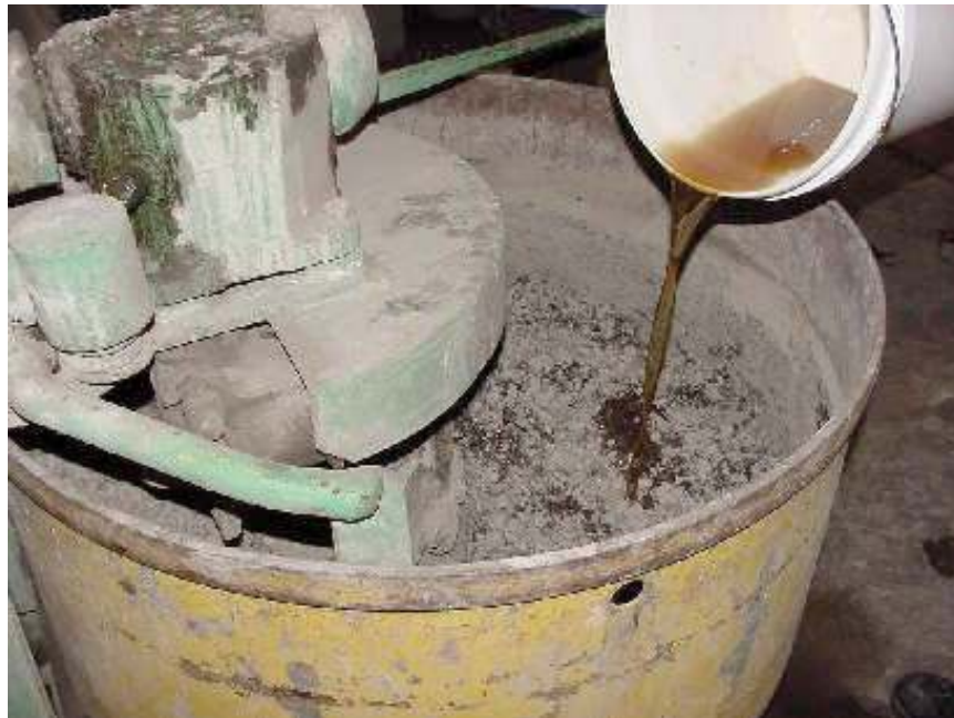
Figure 3.9: Addition of Liquid Component
