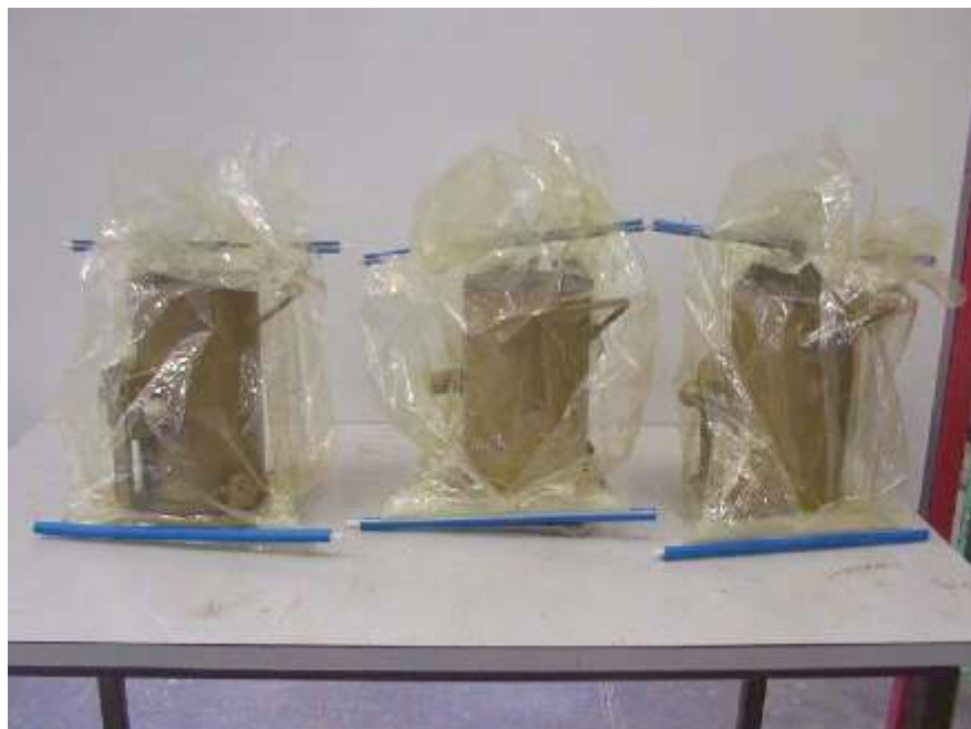
Figure 3.5: Wrapping of Concrete Specimens before Curing (1)
