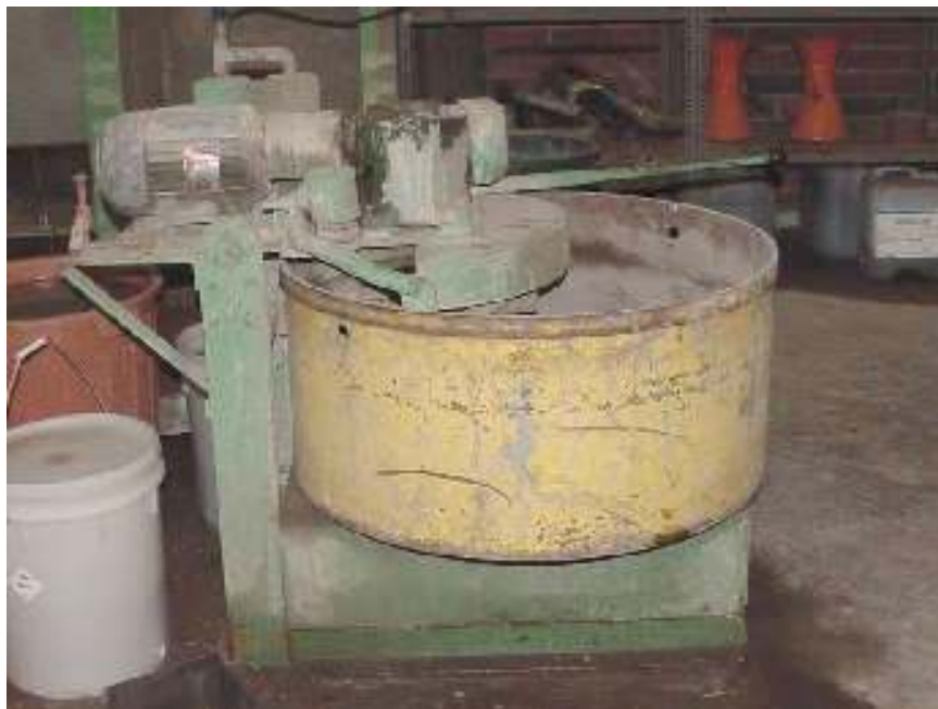
Figure 3.7: Pan Mixer Used for Manufacturing Geopolymer Concrete
