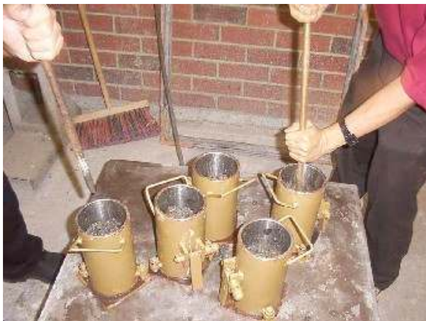
Figure 3.12: Compaction into Moulds
