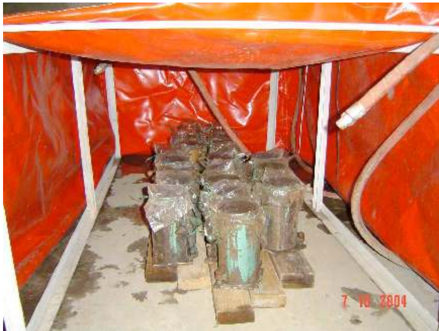
Figure 3.14: Specimens in Steam Curing Chamber
