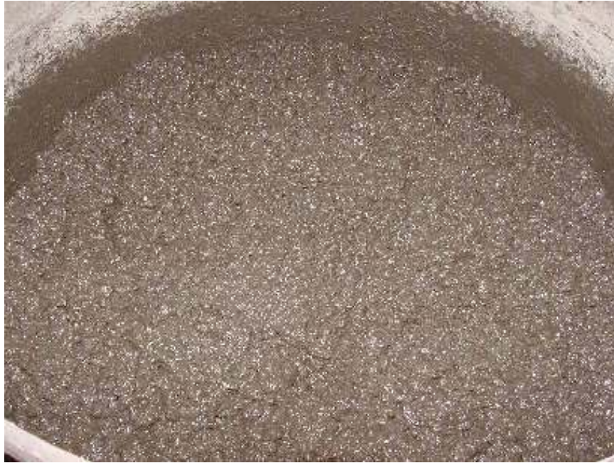
Figure 3.10: Fresh Geopolymer Concrete Ready for Placing
