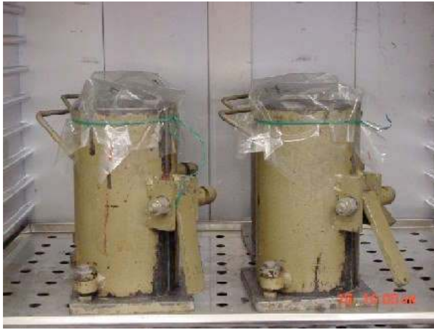
Figure 3.6: Wrapping Concrete Specimens Before Curing (2)
